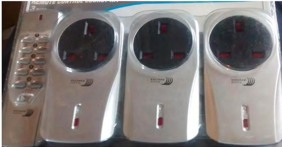
Figure 2. Remote switches for devices – these consume 1 – 1.5W which is often very much less than that from televisions etc on standby.
