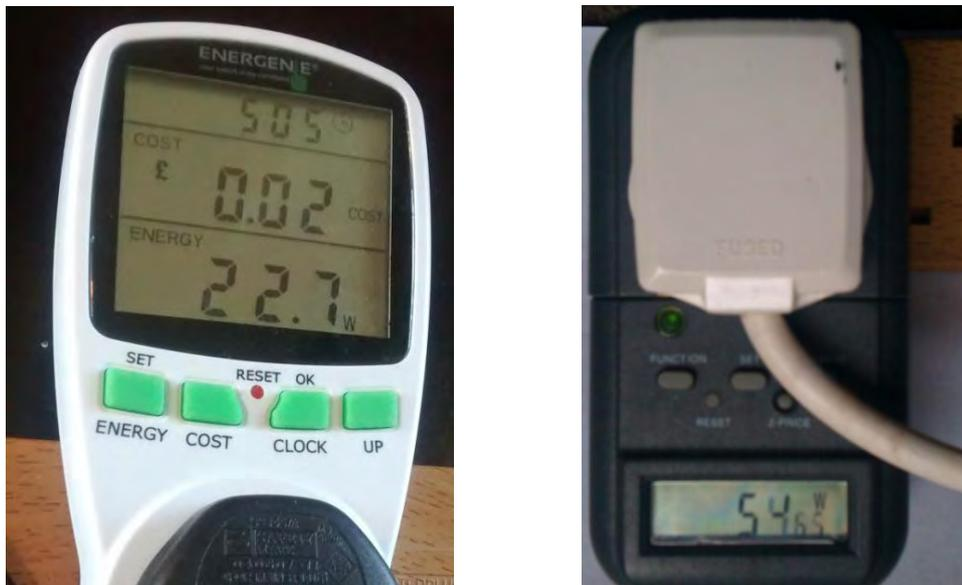
Figure 1. Examples of Energy Meters – the one on the right made by Brennenstuhl is less convenient as the cable can obscure the display. The one on the left is by ENERGENiE.
